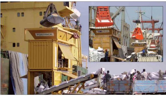
Portpack UK Limited, specialise in the design and manufacture of containerised mobile bagging equipment, to discharge dry bulk materials alongside vessels in destination ports.
